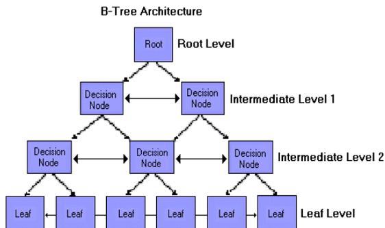
**Figure 1. Architecture of B-tree**
