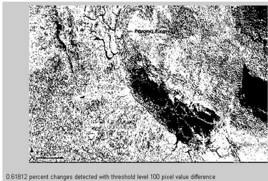
Fig 3.(f) Detection of environmental changes (difference image at threshold 100)
