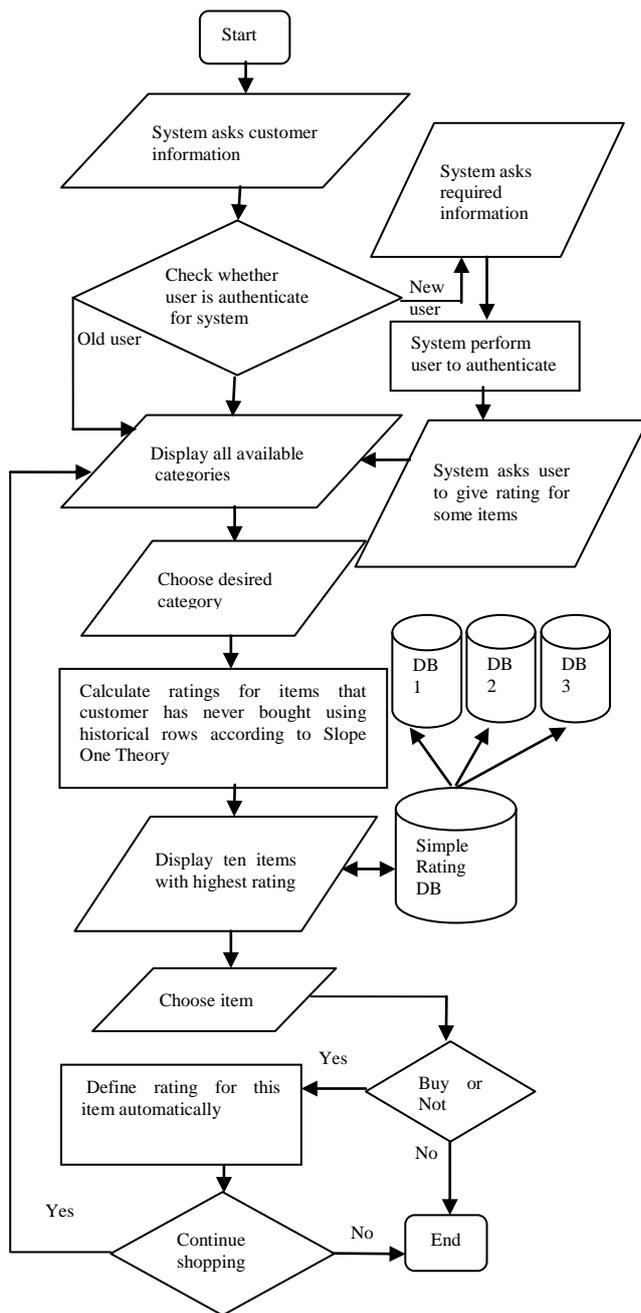
Figure 1: Flow of system implementation
