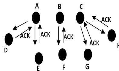
Fig. 2. The parent nodes (A, B, C) send parents request broadcast message and the child nodes send Ack message to their parents using CSMA/CA.
