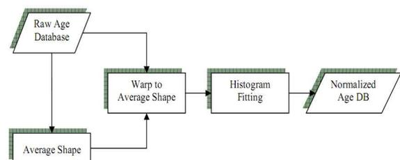
Figure 1. Block diagram of the normalization process
