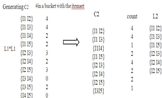
**Figure 4: Generate C2 and L2**
