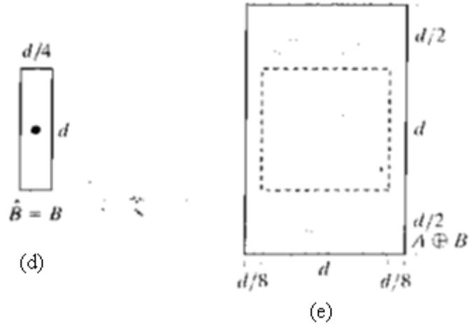
**Figure 2.3 (a) Set A. (b) Square structuring element (the dot line denoted as the origin) (c) Dilation of A by B. (d) Elongated structuring element. (e) Dilation of A using (d). The dotted border in (c) and (e) is the boundary of set A**
