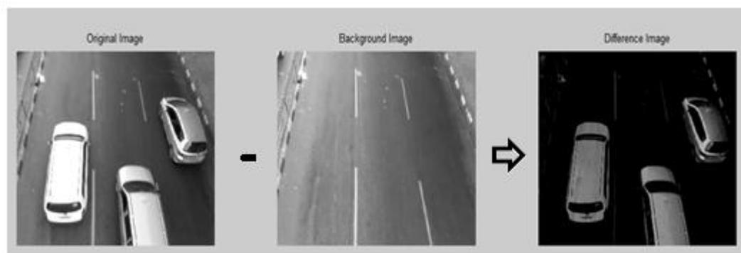
**Figure 4.3 Image Differencing Frame Images by using threshold values**
