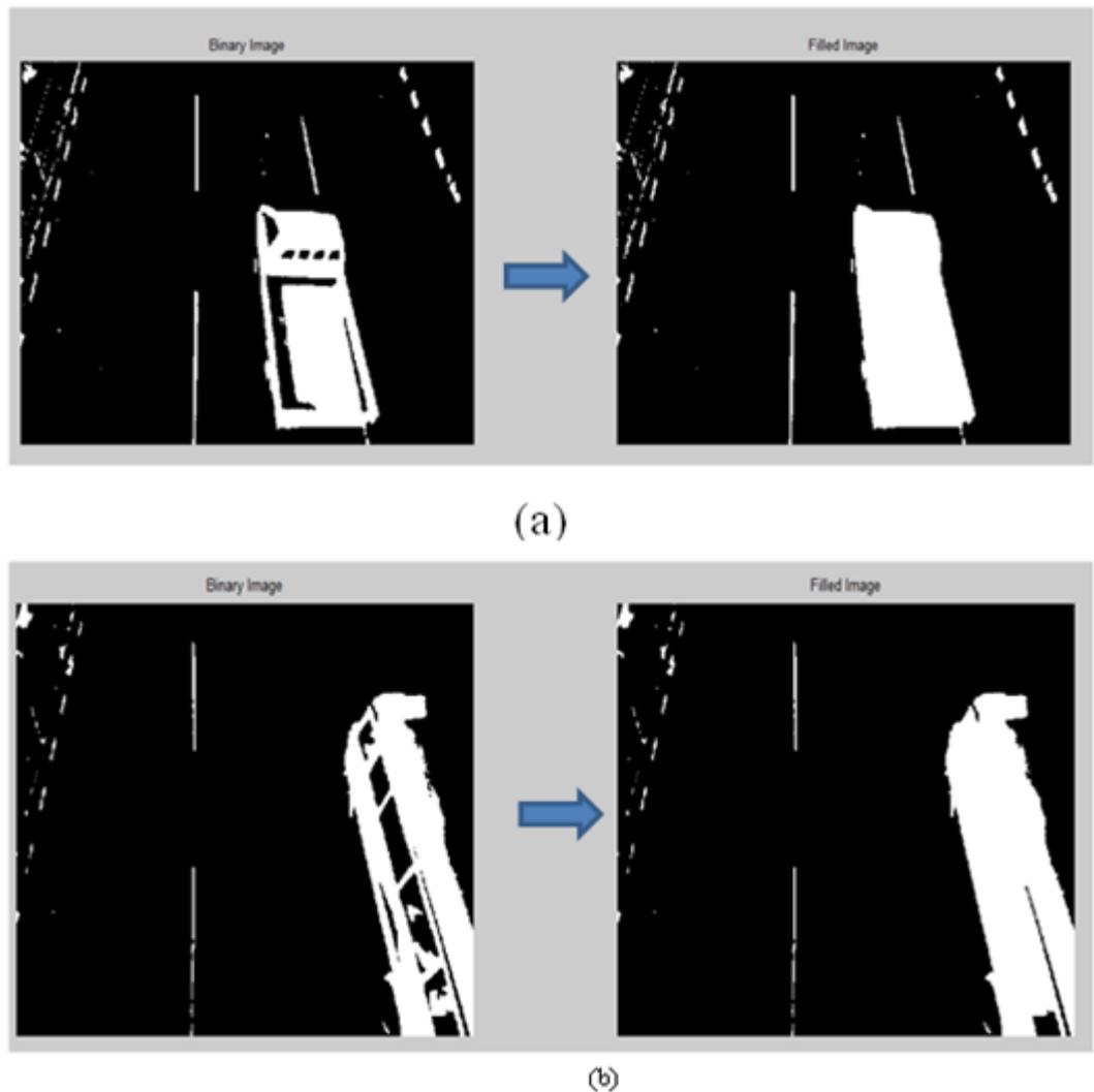
**Figure 4.4 (a) and (b) Filled Image Frames by using morphology filling method**
