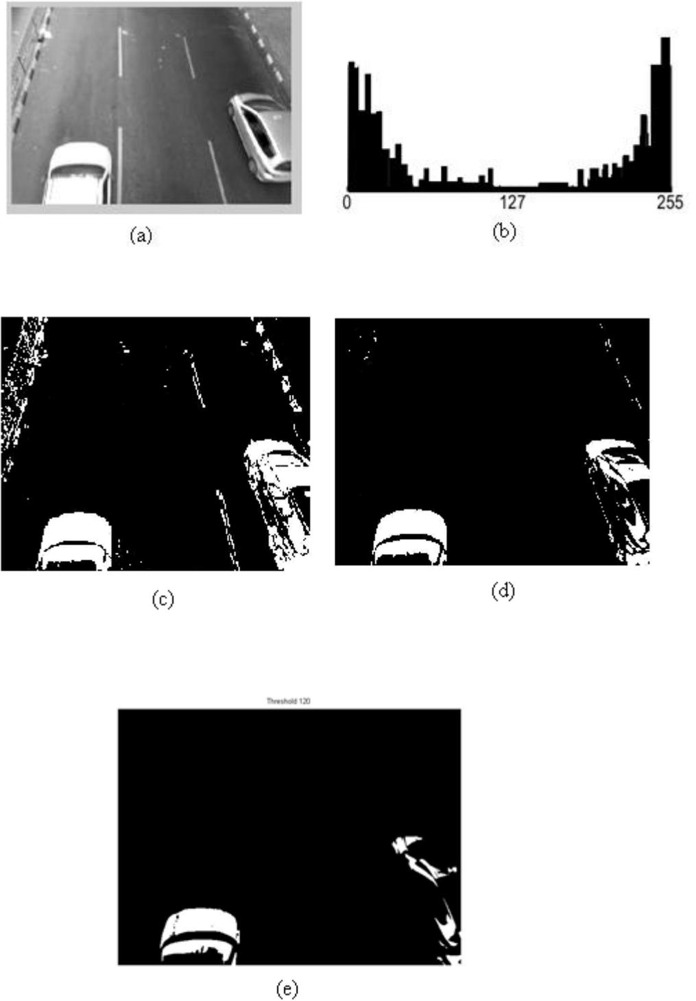
**Figure 3.5 (a) Gray scale image of Cars (b) Its gray level histogram (c) Binary regions for threshold = 20 (d) Binary regions for threshold = 60 (e) Binary regions for threshold = 120**
