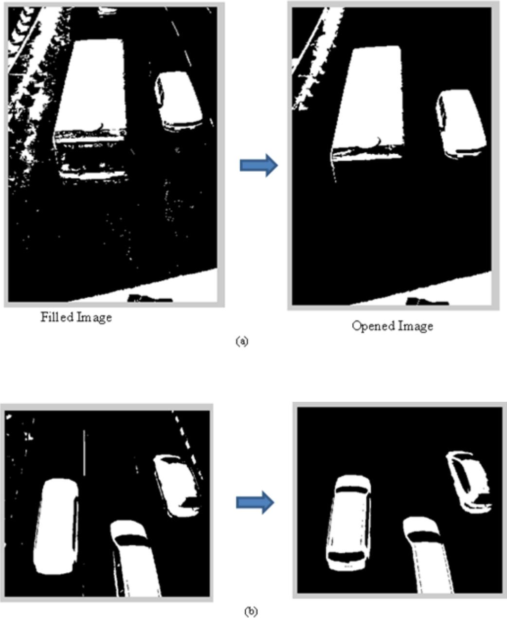
**Figure 4.5 (a) and (b): Removing small structures**
