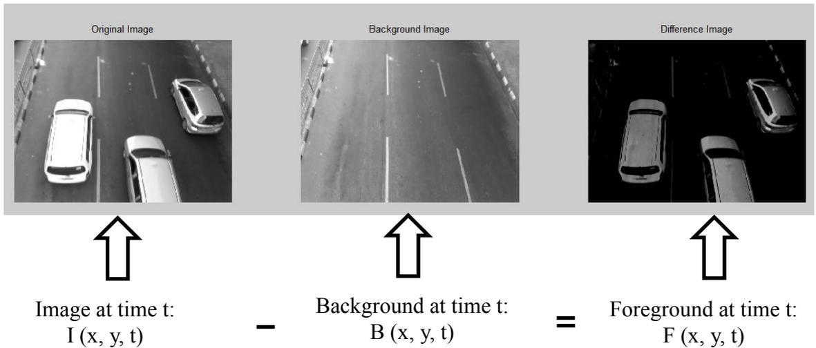
**Figure 3.3 Foreground Object Using Frame Differencing**
