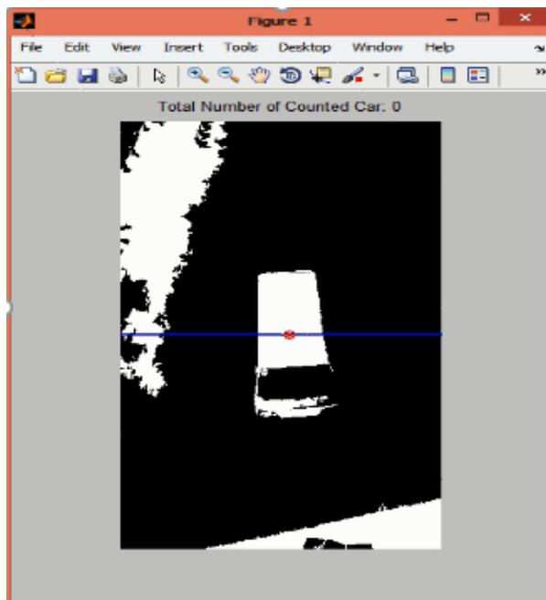
**Figure 4.7 Tags with Red Dot to Object While It Is Passing Through the Line**
