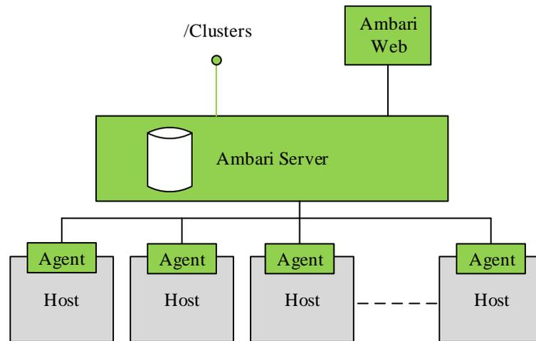
**Figure 4.1 Internal Structure of Ambari Architecture [54]**
