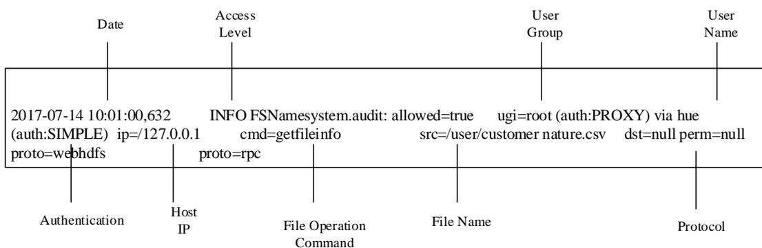
**Figure 4.7 Parameters and Value of a Record in ‘hdfs-audit.log’**
