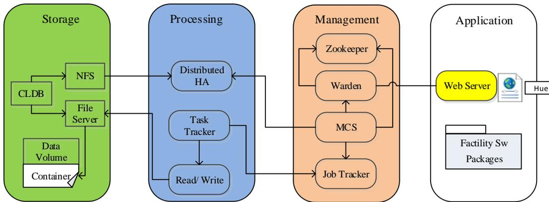
**Figure 6.2 Architecture of MapR Hadoop Platform**
