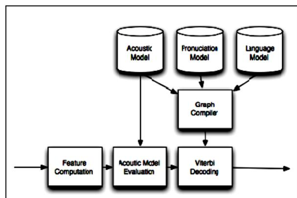
Figure 2. Block diagram of Speech Recognition
