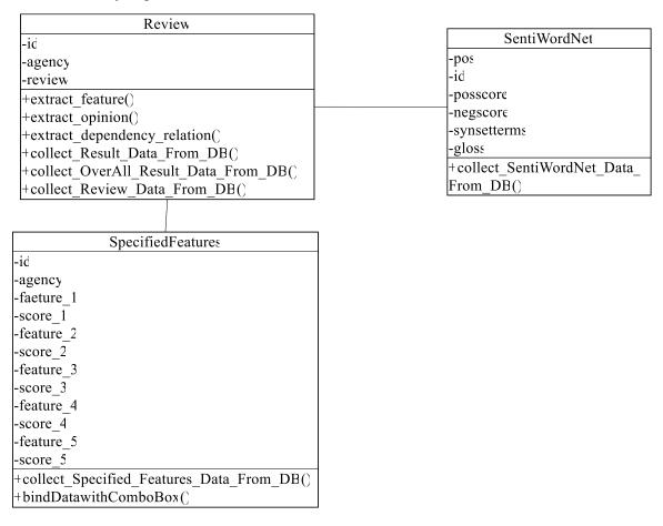
Figure 4.2 Class Diagram for Review, SentiWordNet and SpecifiedFeatures
