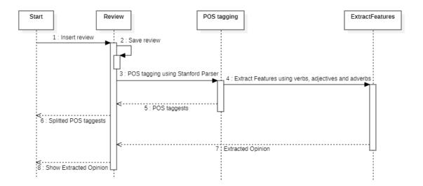
**Figure 4.5 Sequence Diagram for Extracting Opinion Words**
