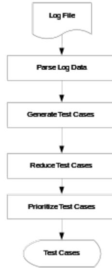
Figure 2. Overall Process of Proposed System
