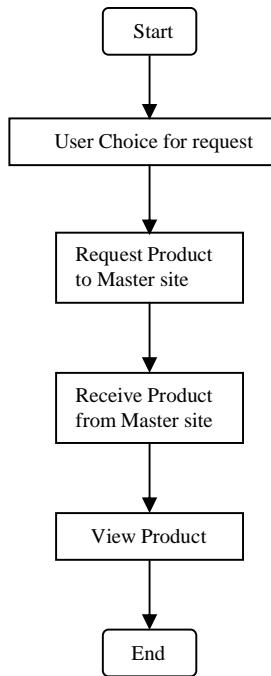
**Figure 4.3(c) Request Process Flow Diagram of Slave Site**
