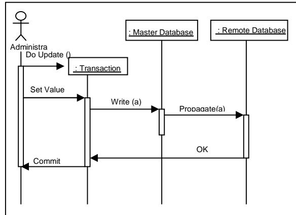
Figure 3.2 Sequence diagram of Eager replication
