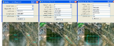
Figure 4-Figure 11. Trajectory setting interface (Waypoint, Line and Area) and Results on realistic maps
