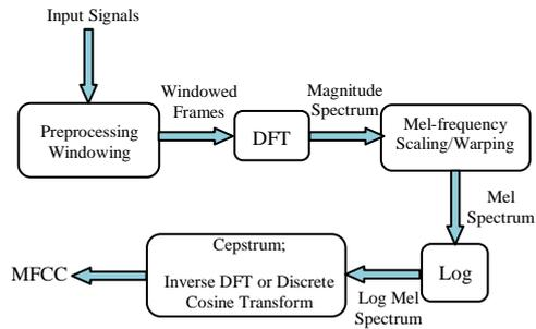
Figure 1. Block diagram for computing MFCCs.
