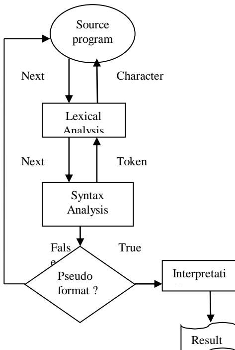
**Figure 1. Flow design of the system**
