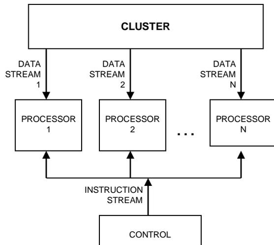
Figure 2: SIMD Parallel Processing
