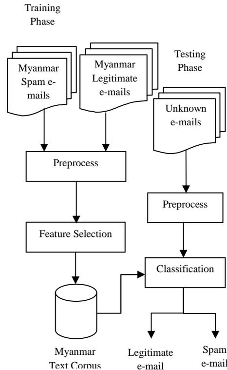
**Figure 2. The System Structure for Training and Testing Phases**
