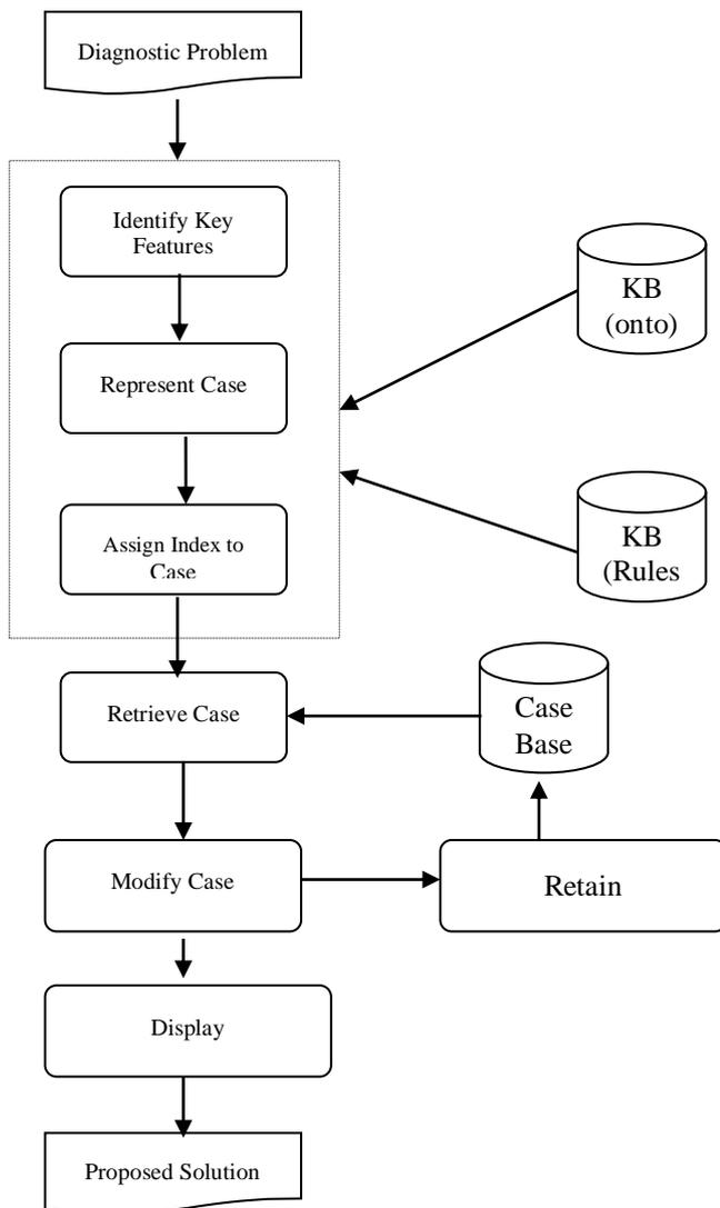
**Figure 2. CBR processes using domain ontology**
