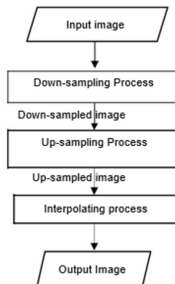
**Figure 1. The general architecture of the proposed framework**
