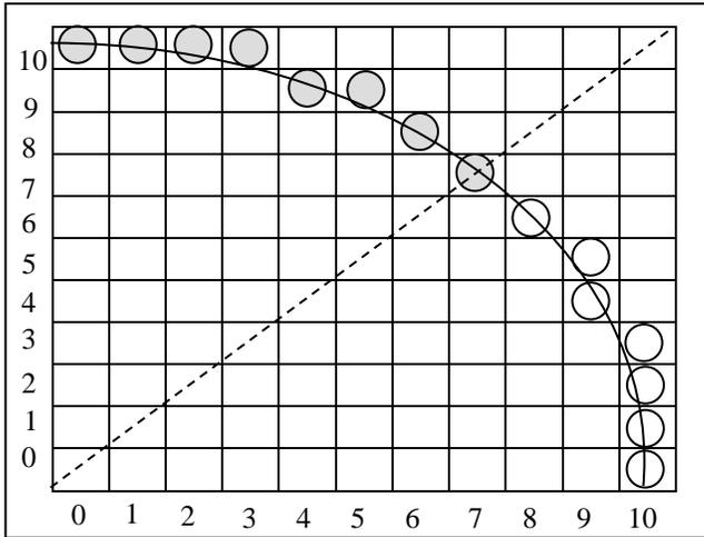
**Figure2.** Calculated point positions (solid circle) along a circle path with  $r=1\text{Km}$  centered on the origin, using proximity detection algorithm. Open circles show the symmetry positions in the first quadrant.
