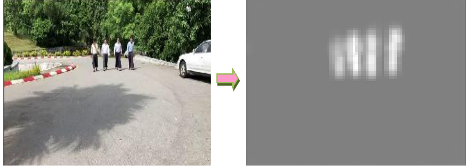
Figure 4.2 Input Image and Result of Segmentation between the Intersection of Target Mask and Prediction Pixels based on ROI Mask
