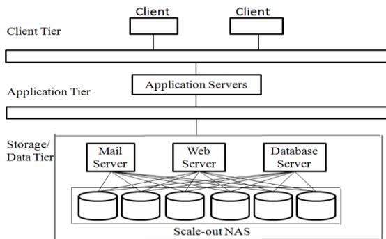
Figure 1. Large scale shared storage system architecture for big data
