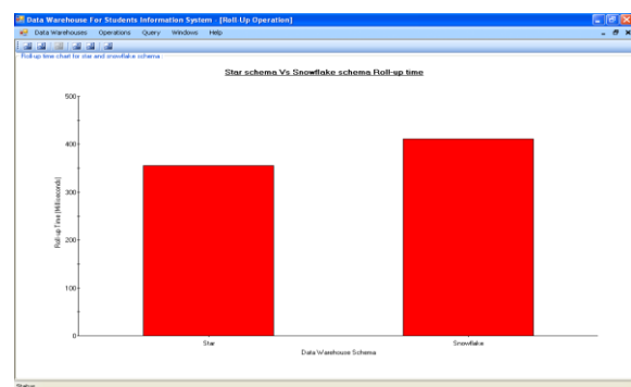
Figure. 9. Comparison of Data Searching Time between Star and Snowflake Schema by using Roll-Up operation
