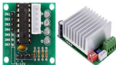
(b) ULN2003A and TB6600 stepper motor driver Figure 7: Stepper motors and stepper motor drivers
