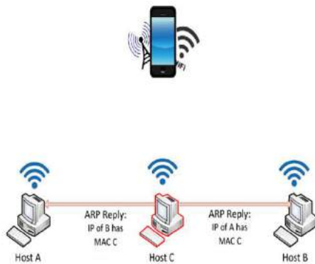
Figure 1. Host C performing ARP cache poisoning attack on Host A and Host B
